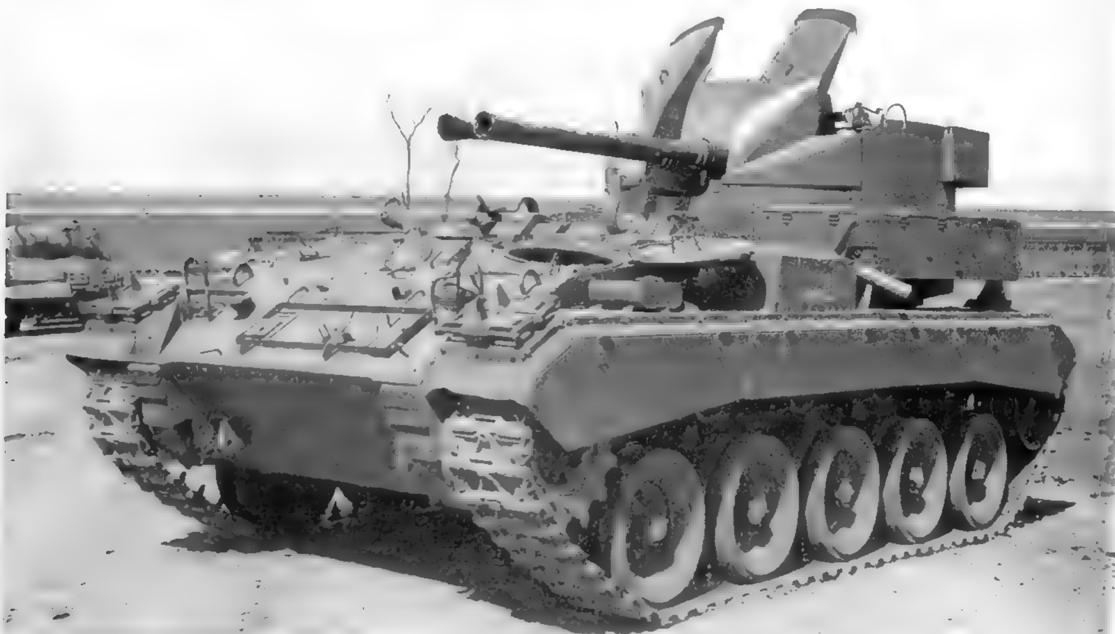
The M19 family's twin 40mm Bofors anti-aircraft cannons were also used with devastating effect against enemy infantry. The vehicle's automotive lineage to the M24 Chaffee is apparent in this April 1949 view of an M19A1. The five road wheels per side were attached to torsion bars. (U.S. Army photo)
